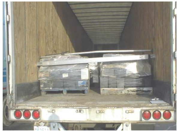
Pic. – Properly blocked back row to prevent movement of the palletized ULAB
