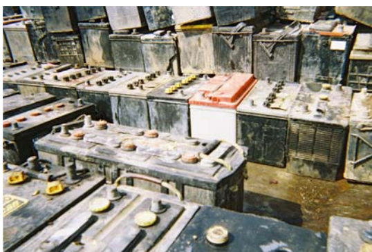
Pic. – A ULAB delivery to Funmetal SA in Venezuela showing protruding terminals and vent caps
