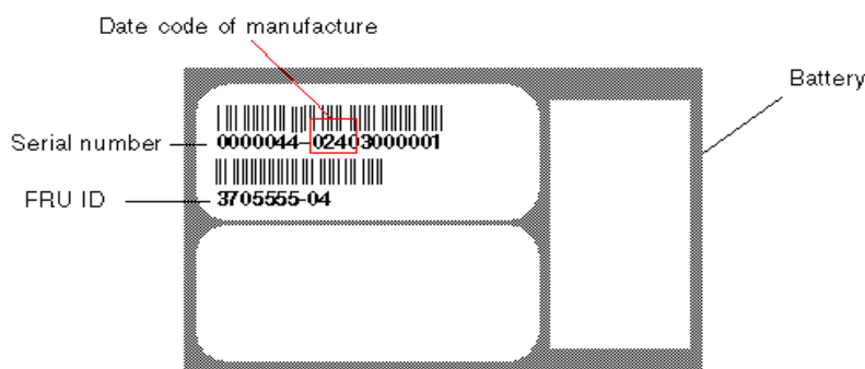
Diag.11 – Date of manufacture - Sun StorEdge 3310 SCSI Array Battery
