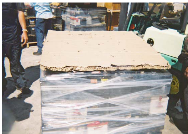
Pic. – The storage yard in Mexico City for Comercializadora de Baterias SA. A sheet of corrugated cardboard is placed on top of the final layer of ULAB.
