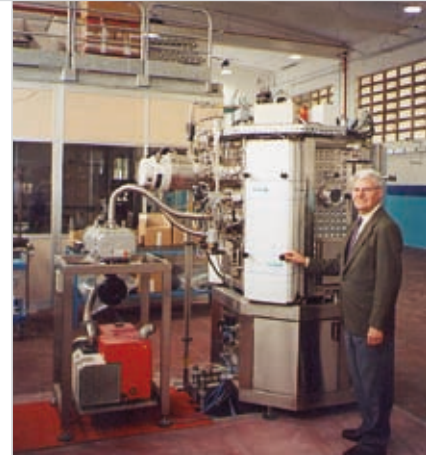
The pilot plant showed that PVD can be used at an industrial scale
