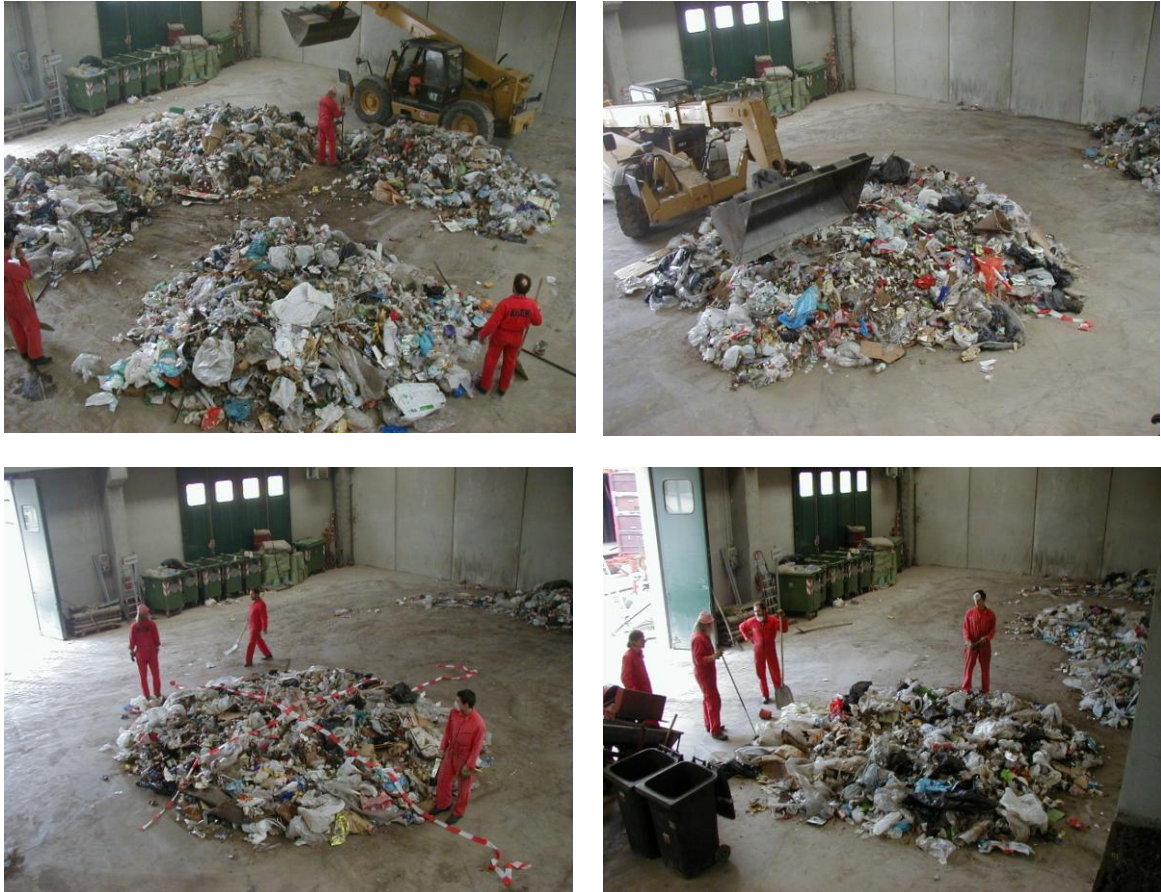
Fig. 5: Sample taking, Option B: Reducing a large waste load by “quartation” to a reasonable sample size to be analysed
