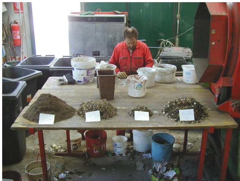
Fig. 8: Combined screen & sorting analysis of the output of a MBT plant: Sorting table, outlet trommel screen (to the right), dryer (in the background)
