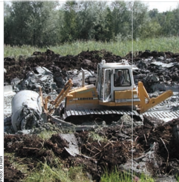
Creation of vegetation-free areas using the tracked excavators originally used in peat cutting
