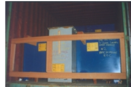
Photo : Transport unit bracing
